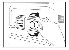
The operating temperature is regulated by the temperature control.
